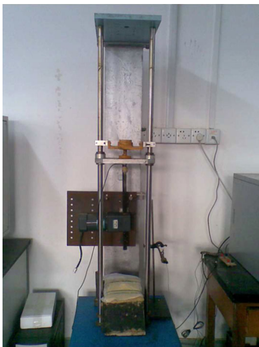
Figure 1. Homemade dynamic puncture tester. [Color figure can be viewed in the online issue, which is available at wileyonlinelibrary.com .]
